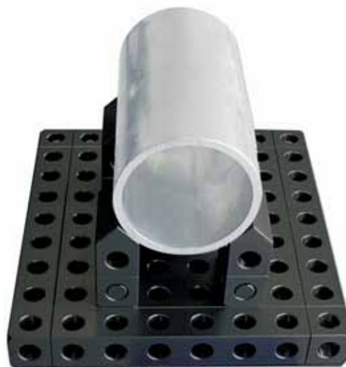
Arrange 2 delta blocks in a V to support round parts
